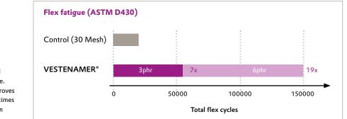
The graph shows significant improvement in flexibility and contributes to a longer lifetime. VESTENAMER<sup>®</sup> addition improves total flex cycles from 7 to 19 times when dosage is increased from 3 to 6phr.
